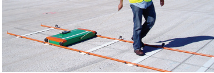
Figure 12. Pulling the MIT Scan device along the rail system.
