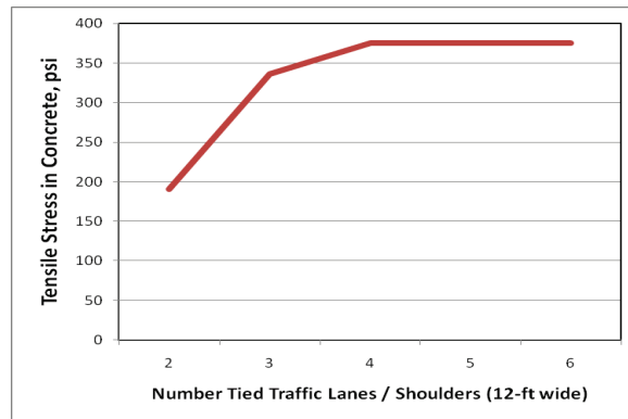
Figure 54. Tensile stress in the concrete slab built over a CTB vs. the number of tied lanes/shoulders.
