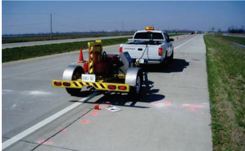
Figure 17. FWD testing of one of the sections at the Missouri test site.
