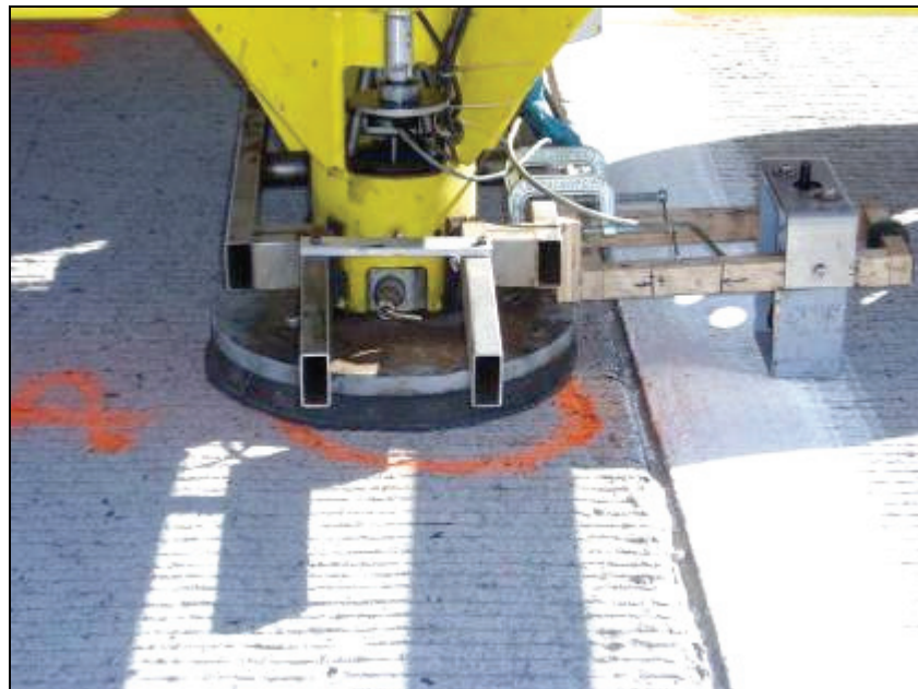
Figure 10. Close-up of FWD load plate and side sensor.
