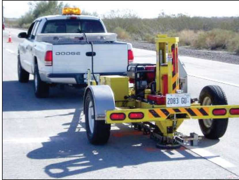
Figure 9. FWD configured for longitudinal joint LTE testing.
